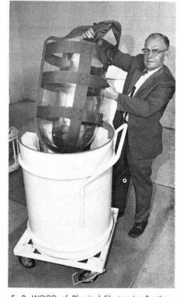
E. R. WOOD of Physical Electronics Section displays his new safety system for moving and handling large, glass, laboratory bell jars. Converted A/N can has wheels, handle, and foam cradle inside.
